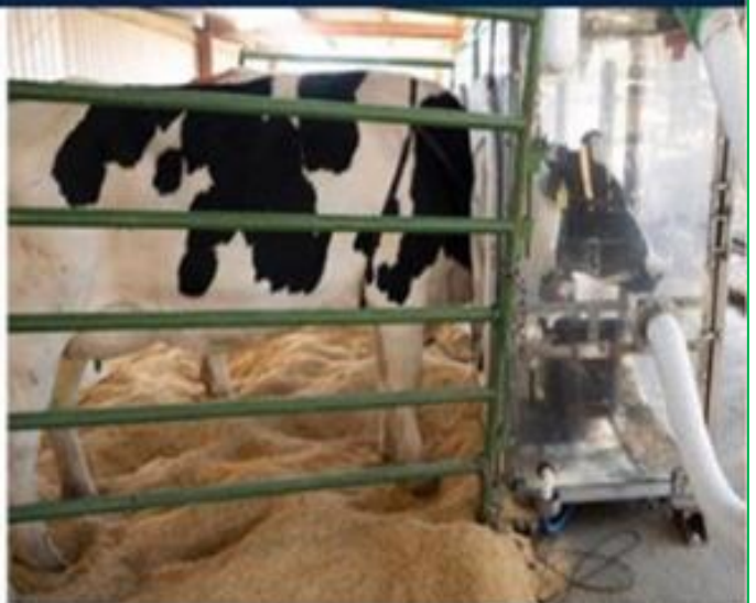
The plastic chambers help measure the amount of gases cows release from their stomach more precisely. Each year, one cow can belch 220 pounds of methane, which is 28 times more potent than carbon dioxide. 15 Karin Hin
